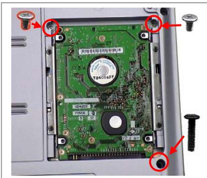
**Step 8.** Using the enclosed magnetic screwdriver, reinstall the three (3) previously removed screws. **CAUTION!** Be careful not to drop screws into the inside of the unit, and be careful to use the correct screws, as shown in the picture. Do not over tighten the screws!
