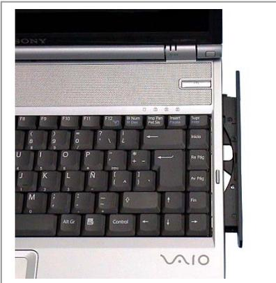
**Step 1.** Power on the PC, eject the CD/DVD drive tray by pressing the button on the drive door. Next, properly turn off the PC, leaving the tray ejected.
