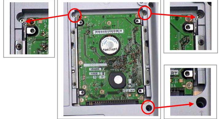
**Step 5.** Using the enclosed magnetic screwdriver, remove the three (3) screws as indicated in the picture. **CAUTION!** Be careful not to drop screws into the unit
