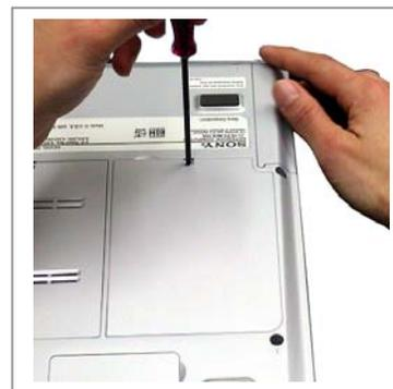
**Step 9.** Using the enclosed magnetic screwdriver, reinstall the external door and screw. Return the old CD/DVD drive to Sony following the included shipping instructions.
