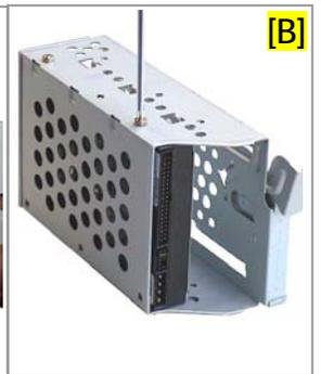
**Step 7.** [A] Slide New Hard drive inside bracket with all holes in alignment. [B] Reinstall the four (4) screws previously removed, securing new drive into the bracket.
