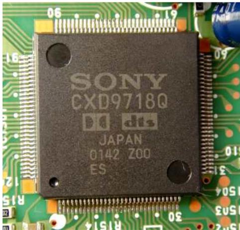
*The latest expression of decoding accuracy is Sony's CXD9718 Large Scale Integrated circuit (LSI).*
