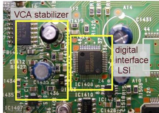
*The combination of the Digital Interface LSI and Sony's VCA stabilizer makes for an uncommonly consistent internal clock, for uncommonly accurate regeneration of digital input signals. So jitter is effectively suppressed.*
