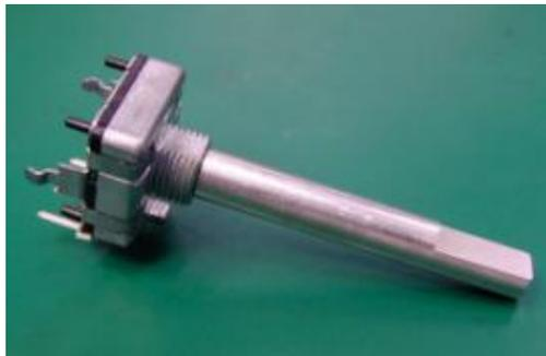
*Sony improves the tactile quality of the STR-DA4ES and DA7ES with this metal-shaft rotary encoder.*
